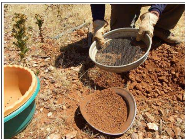
Figure 33, showing the 5mm metal sieve (steel wire, aluminium body) and the stainless-steel collection plate. The items were wiped clean between samples with cloth.
