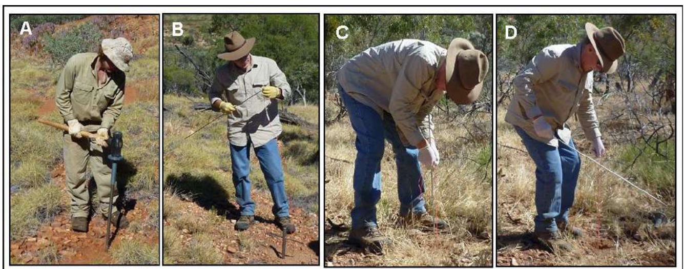
Figure 29, the process of implanting a GORE module. (A) Making hole with heavy sledge hammer, rod and collar.
